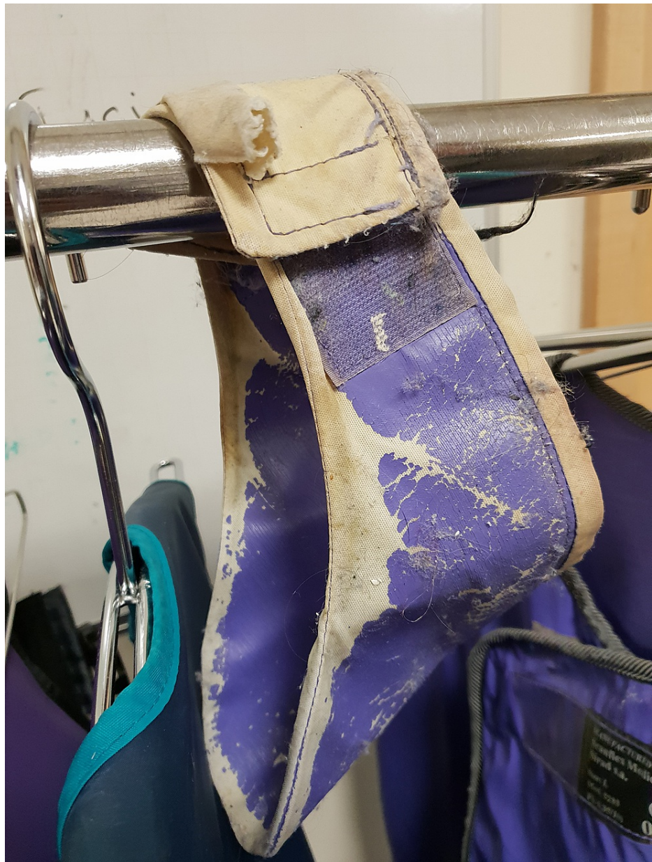
FIGURE 9: Photograph of the poor condition of thyroid shields available to staff.
